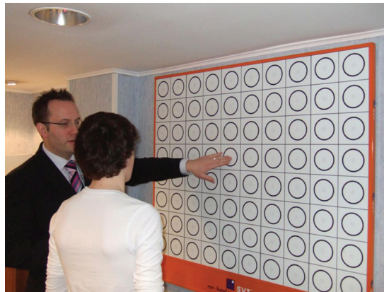
The SVT board contains 80 touch-sensitive LED lights
